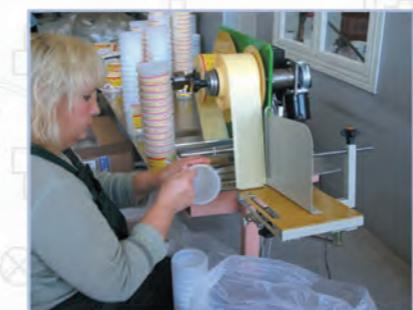
This modification is additionally supplied with thermal printing device which allows automatically print digital or literal information on labels. Information is printed on label at specified place by hot stamping. Printing three-rows matrix has the changeable symbols 14x30 mm size.
