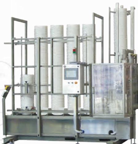
The station is equipped with control system based on PLC Siemens with Touchscreen and can work offline out of system.
