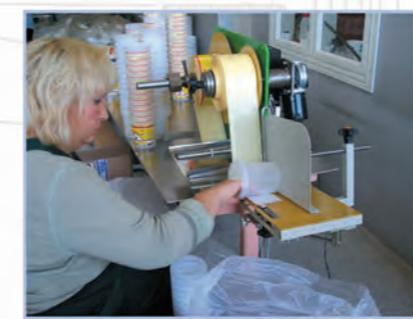
Machine is used for automatic separation self-adhesive labels from substrate and its delivery on special table for fast and precise gluing on different tare (cans, buckets etc.) as well as on different things or packages.
